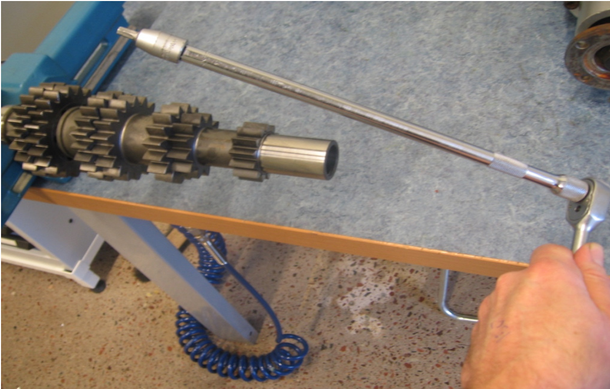
Use a 6mm Allen socket on a long extension
