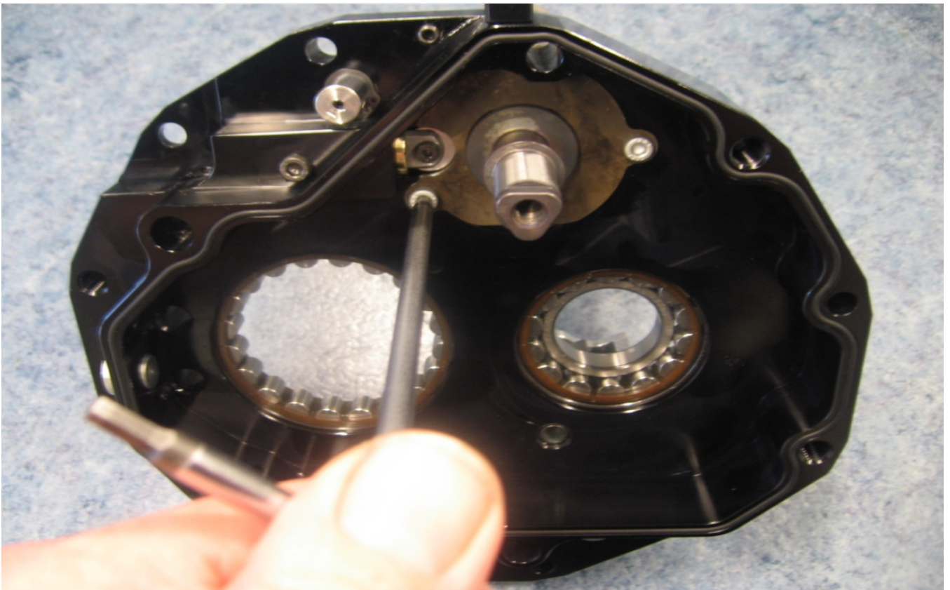
Remove the two M5 screws from the stop guide plate
