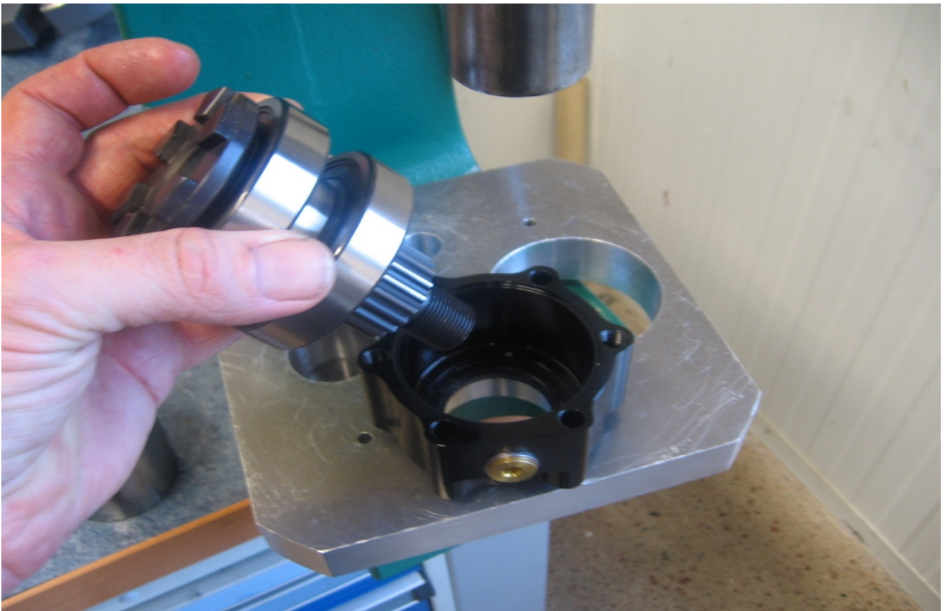
Press in the flange assembly to the bearing housing.
