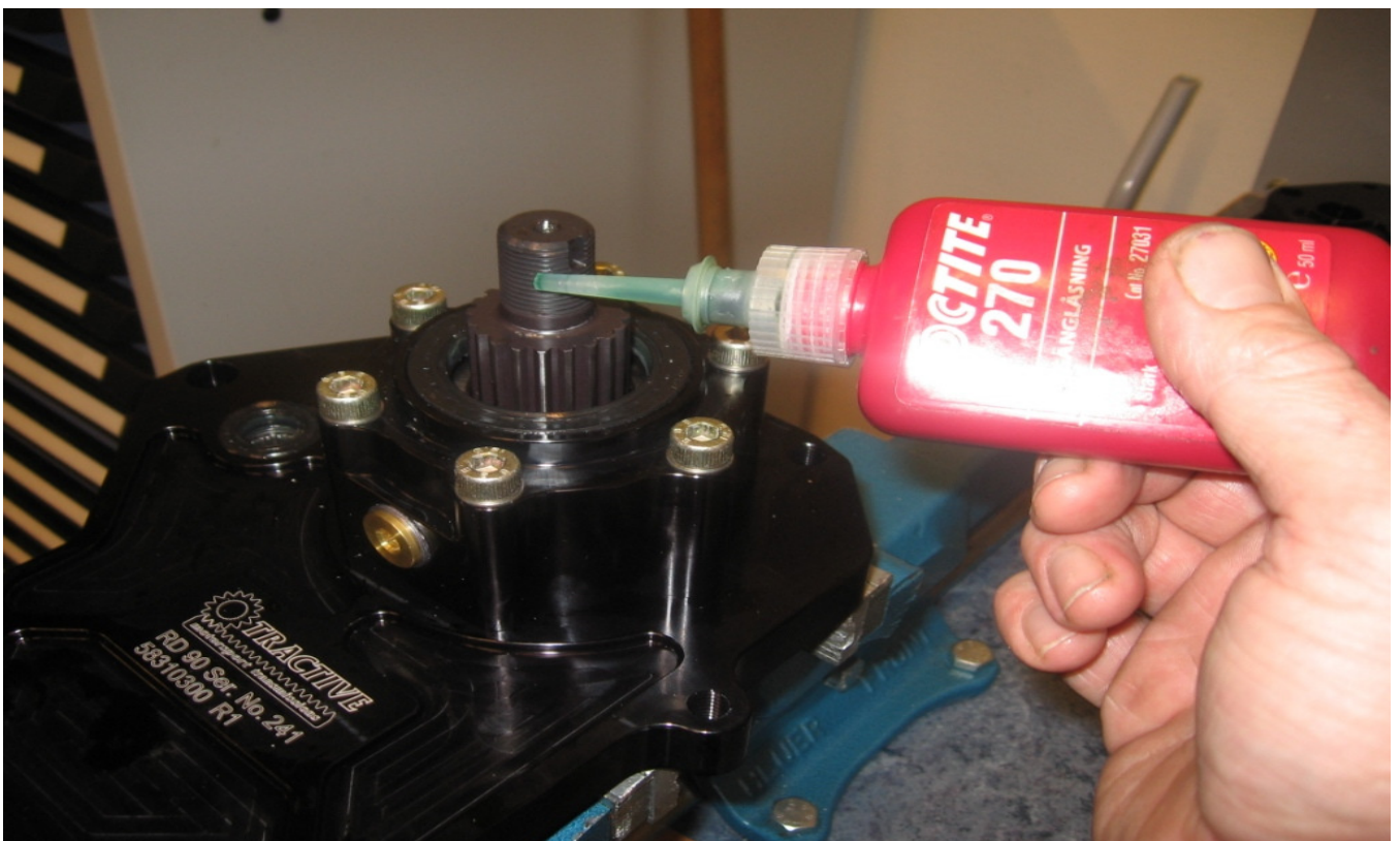
Apply 270 Loctite to the threads of the output flange (make sure threads are free of oil and grease)
