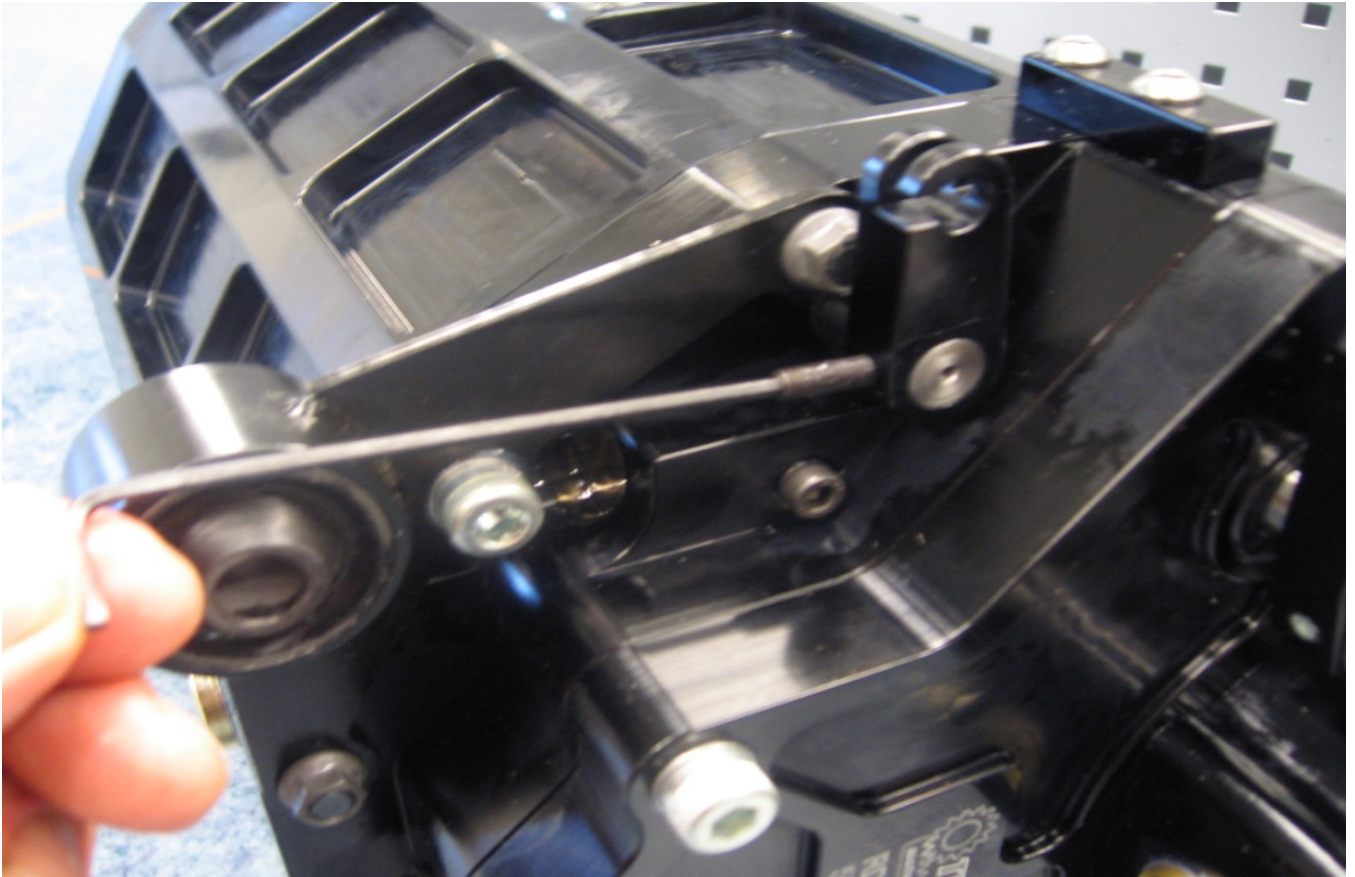
Fit the neutral reverse arm, (2,5 mm Allen key)
