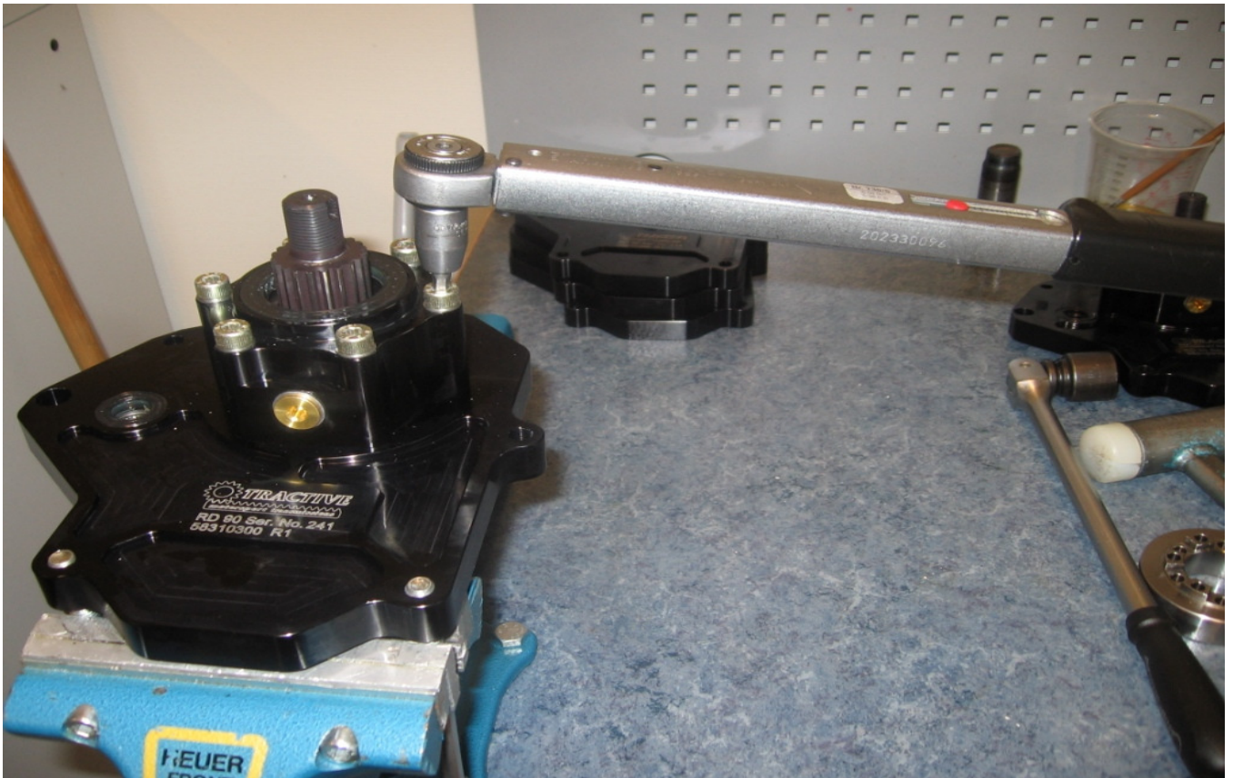
Torque the six bolts to 36 Nm
