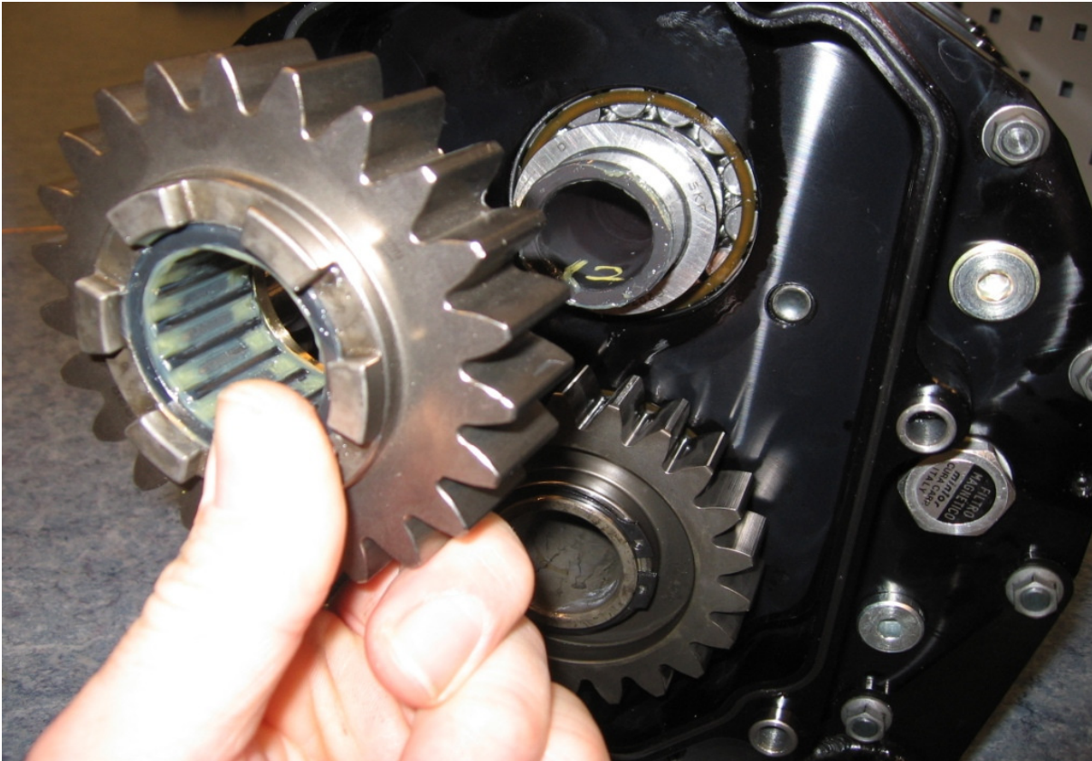
The upper drop gear is not fixed on the shaft and can be removed with the bearing.
