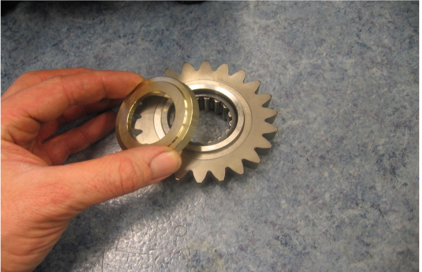
Fit bearing and brass thrust washer
