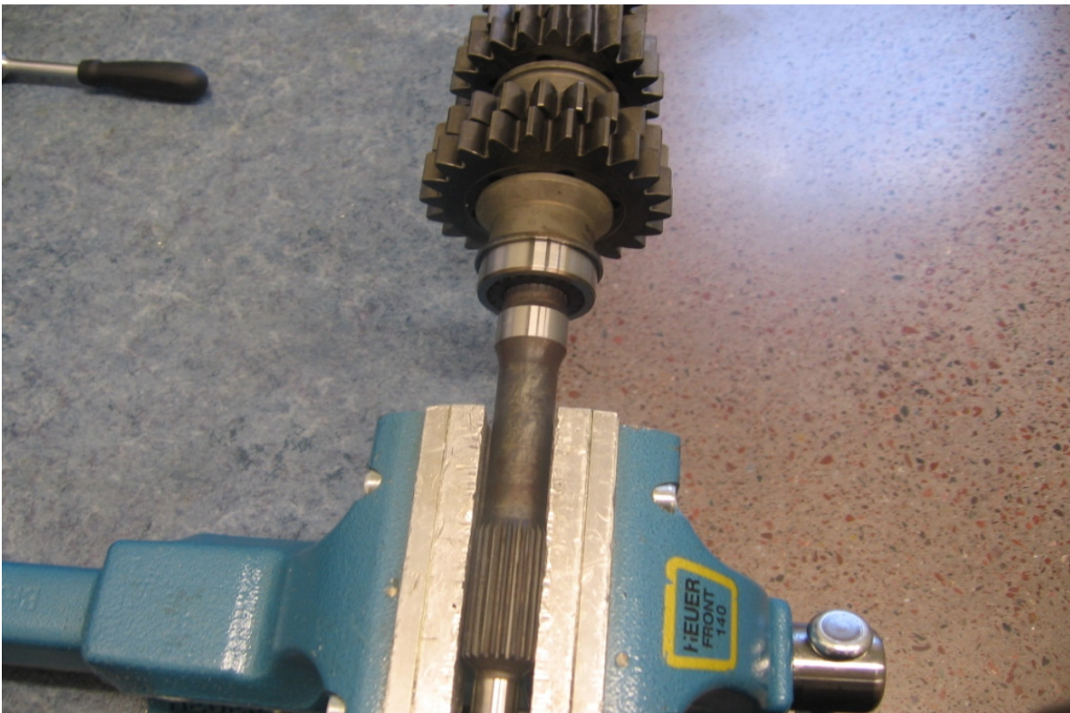
Hold the clutch shaft in some soft jaws.
