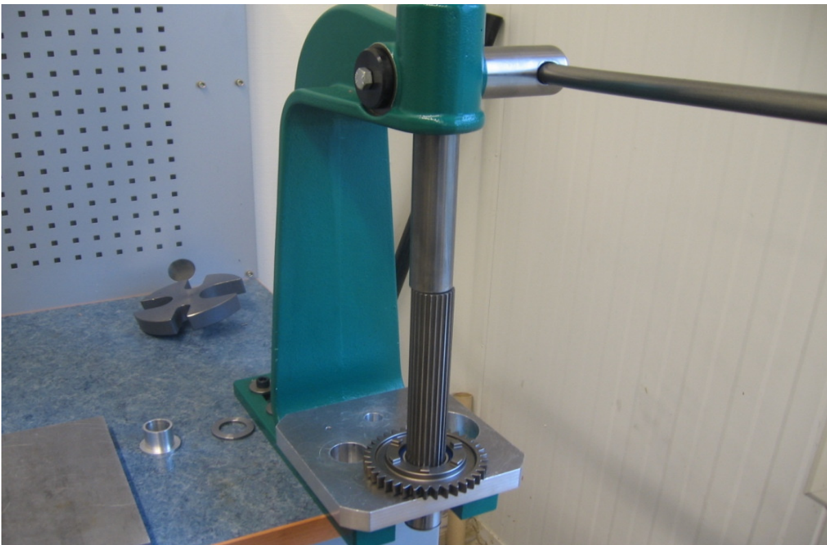
Press mainshaft through the reverse gear.
