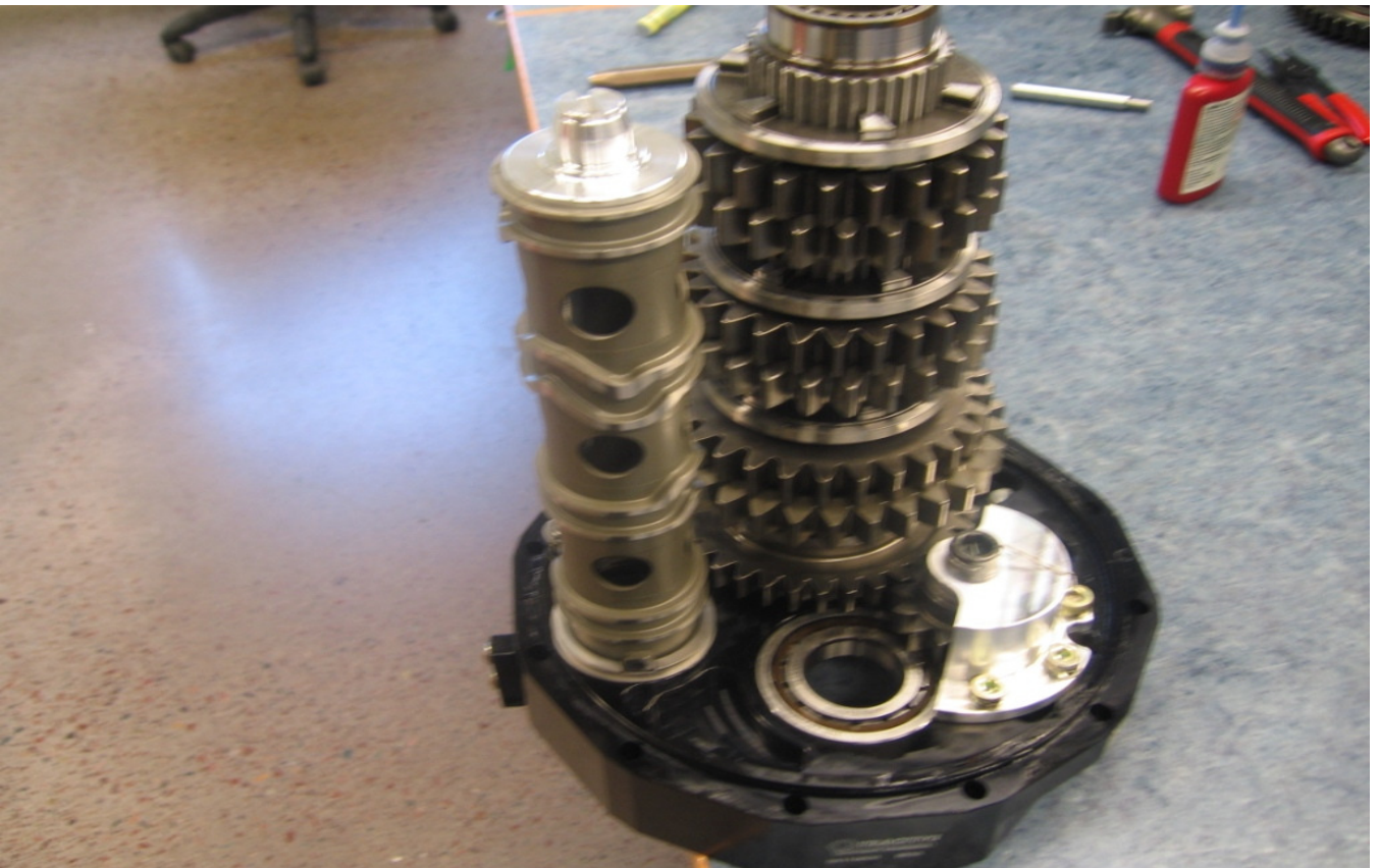
Fit the mainshaft into its bearing engaging the reverse idler.
