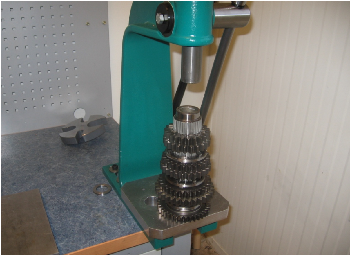
Support the reverse gear on the arbor press
