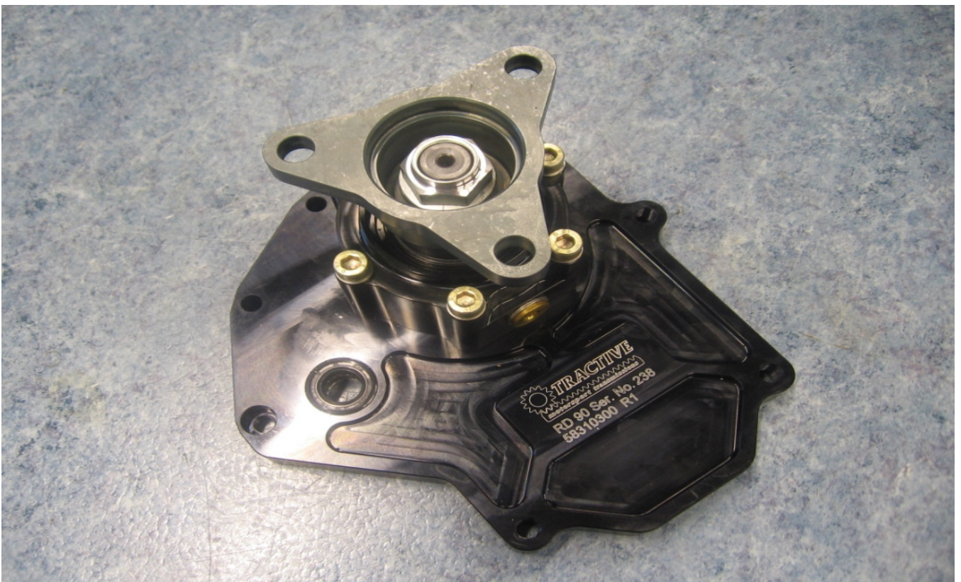
Drop gear cover assembly.
