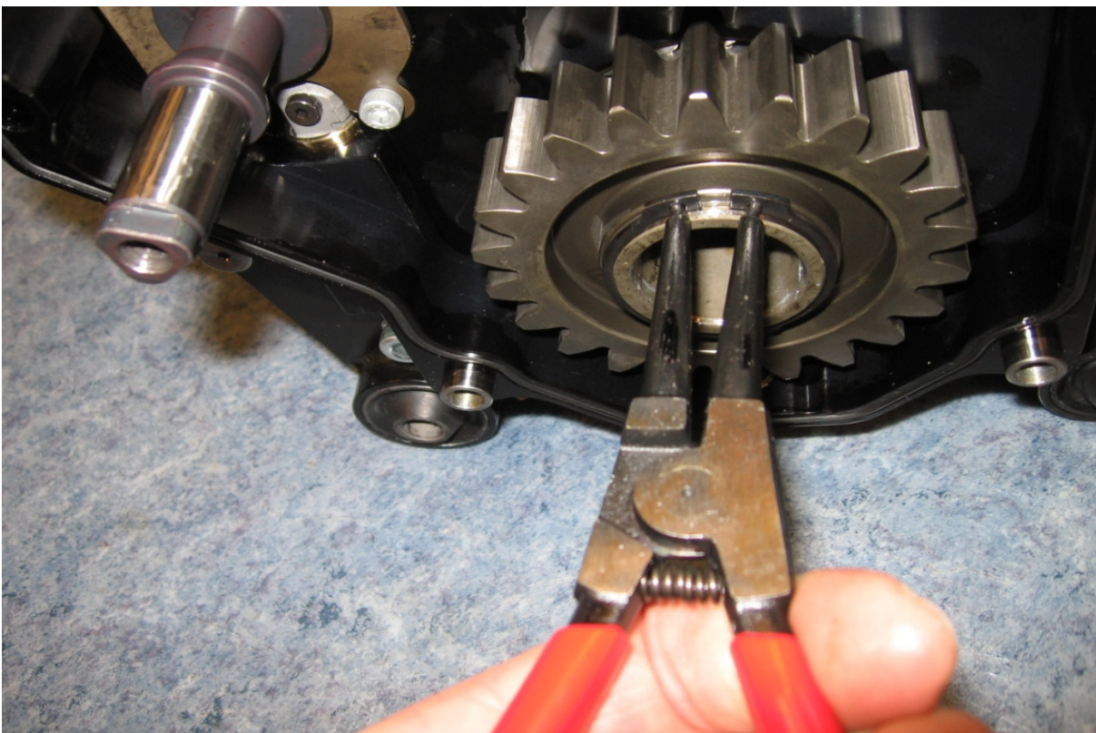
Lower drop gear is held in place by a circlip
