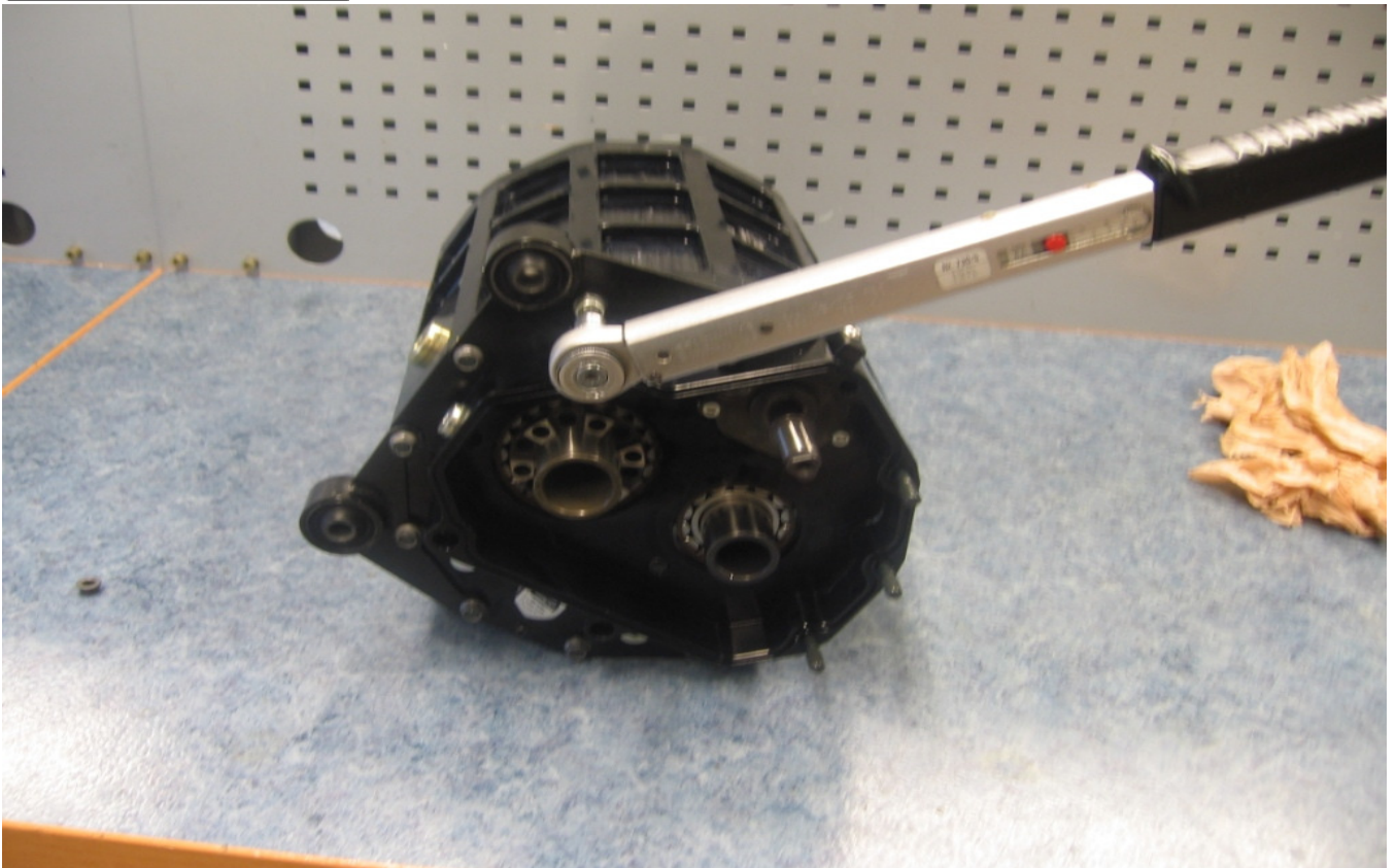
Torque “K” nuts to 20 Nm & Allen screw to 30 Nm
