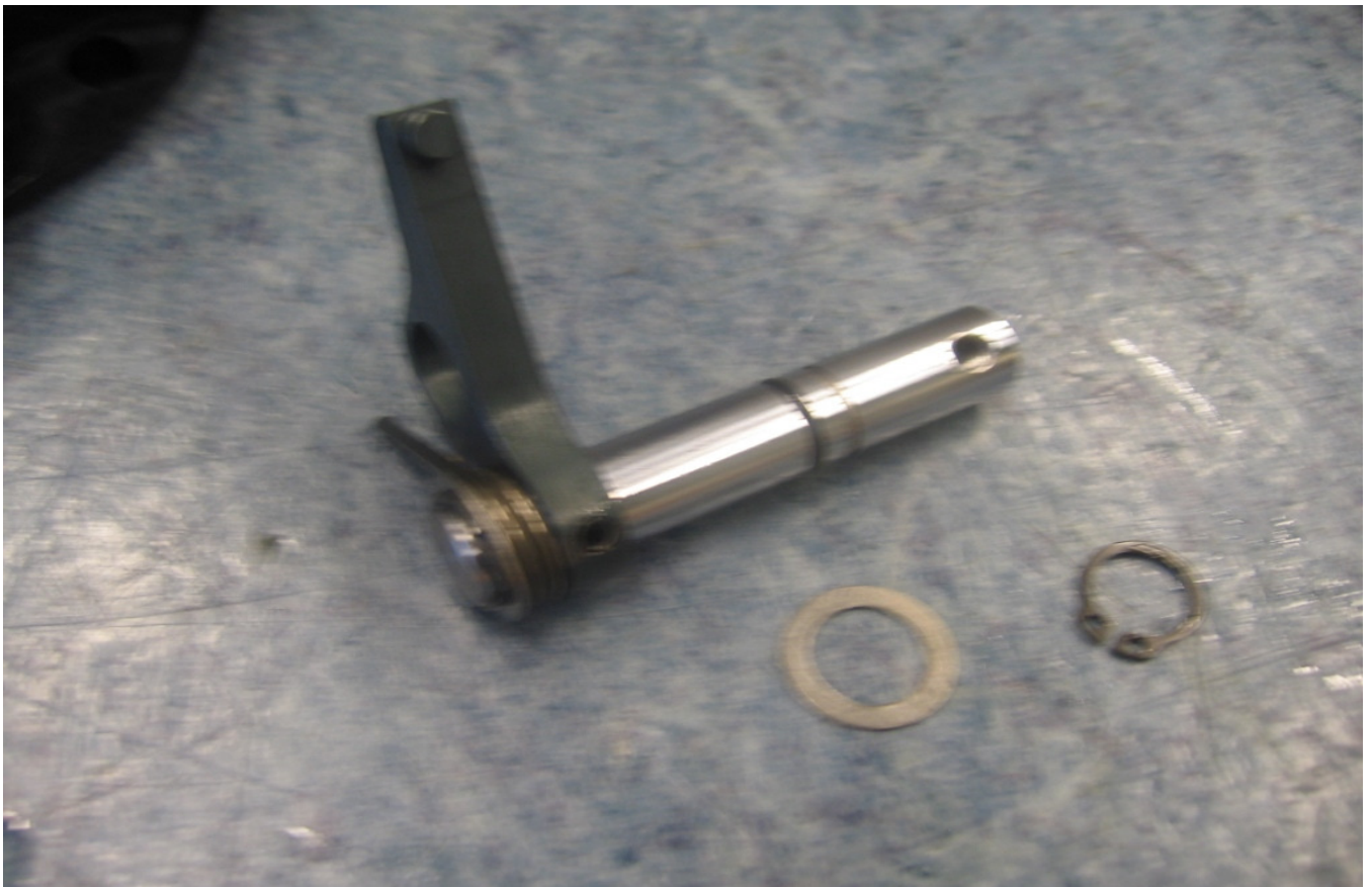
Remove circlip from neutral reverse axle.
