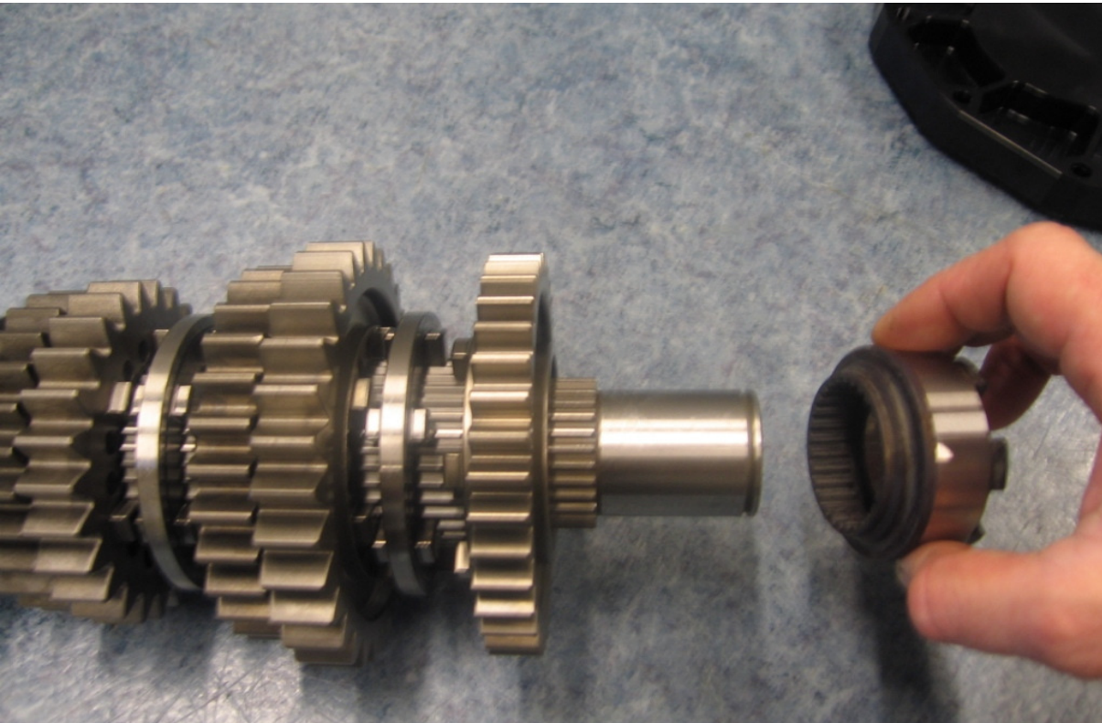
Remove the bearing hub from the end of the shaft, (it may still be in the cluster housing)
