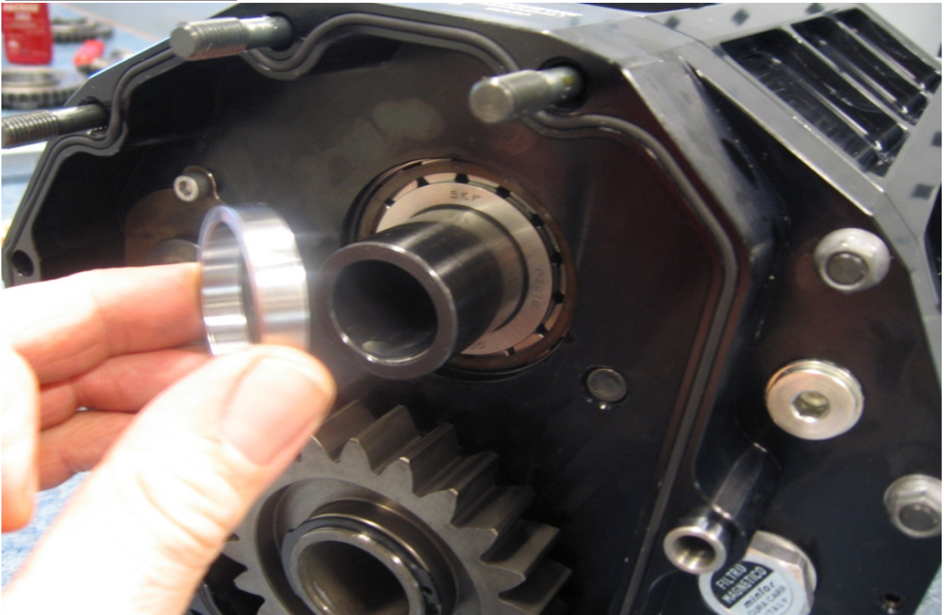
Fit the 8mm steel spacer to the upper shaft
