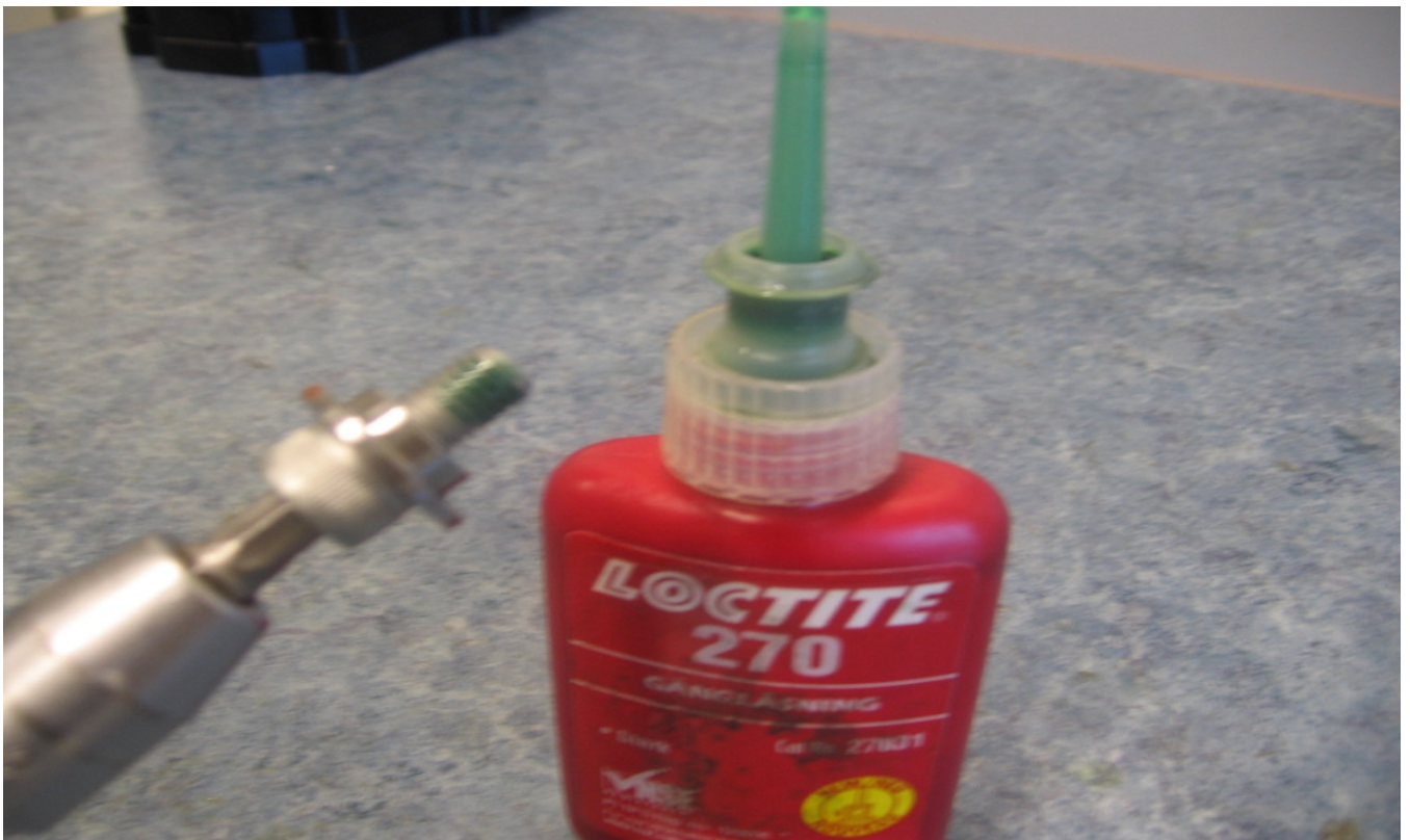
Apply Loctite 270 to the clutch shaft retaining bolt.
