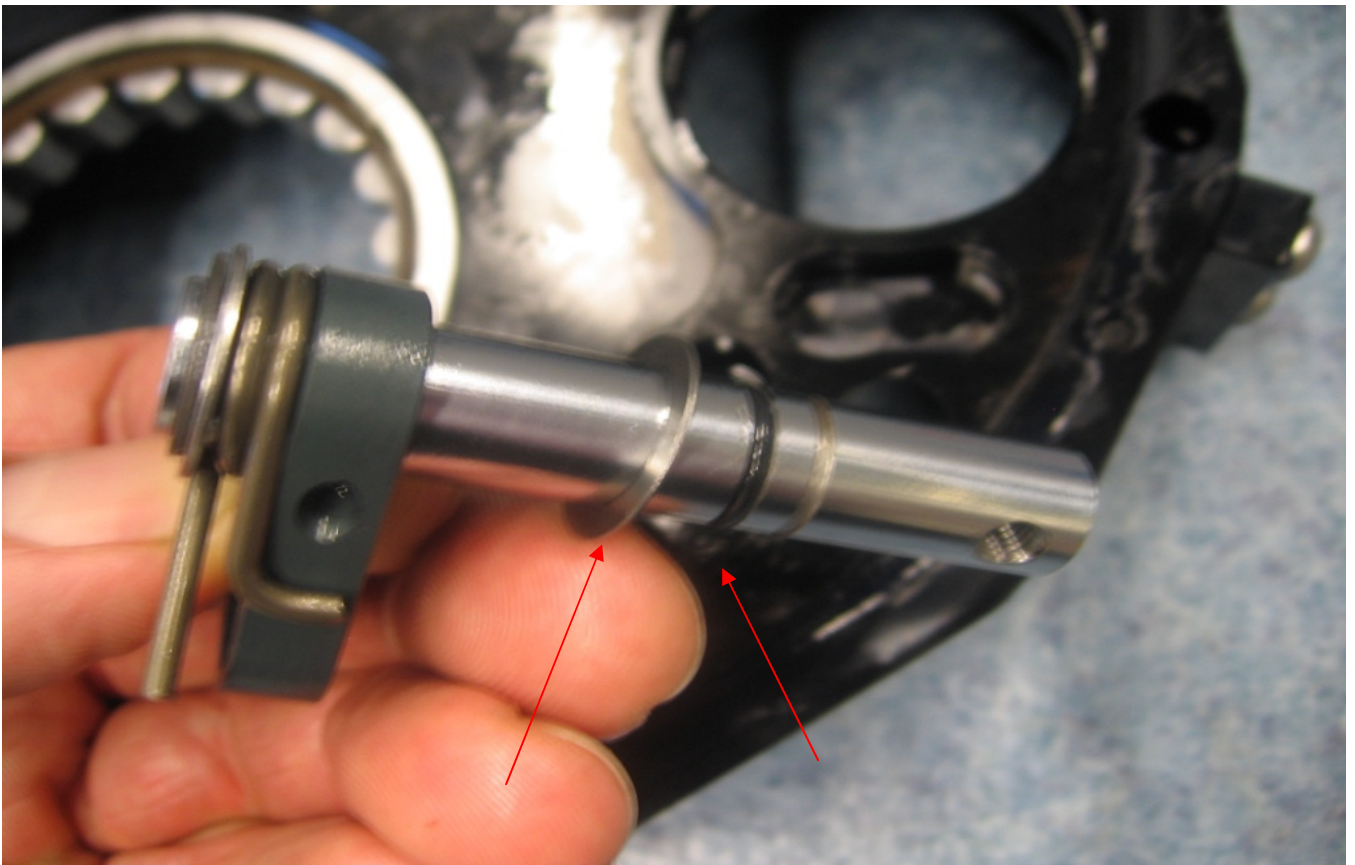
Neutral reverse axle, note "O" ring (9 x 1,5) and position of 0.5mm spacer.
