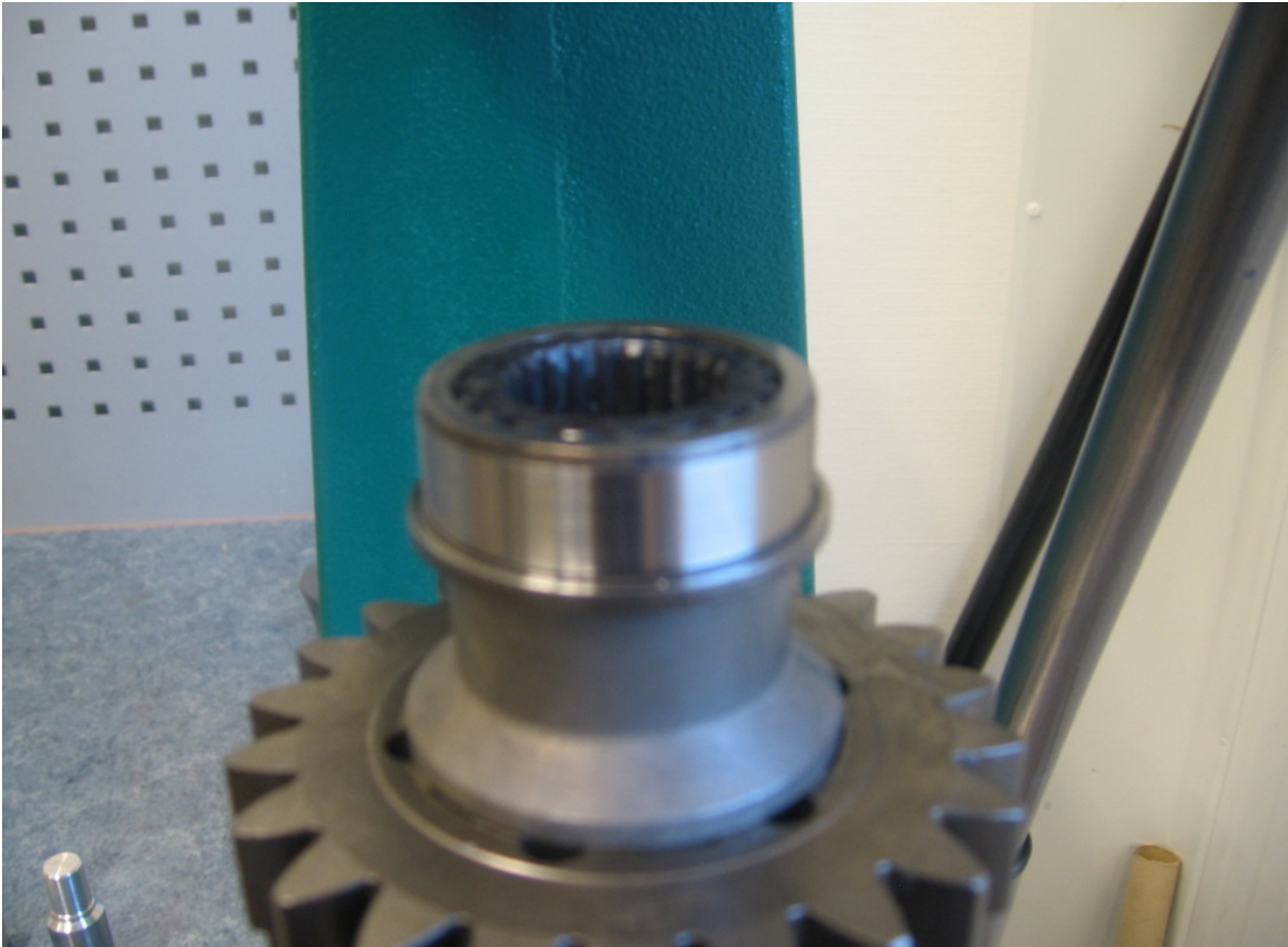
The race should be flush with the end of the shaft.
