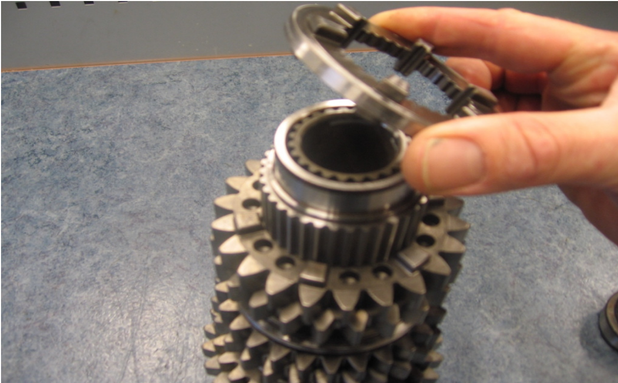
Lift off the 6 th gear dog ring, Note- only one side of this dog ring is used
