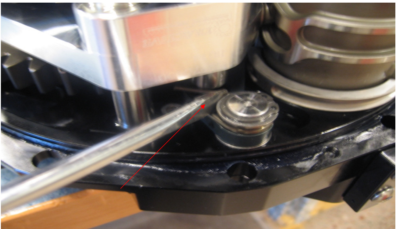
The inner rod should be placed just above the spring then using a screw driver push the spring to the other side of the rod then push down the rod.
