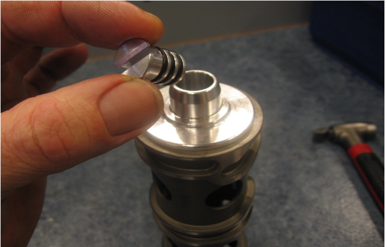
Potentiometer drive, do not remove this part or turn it otherwise the display will have to be reset.
