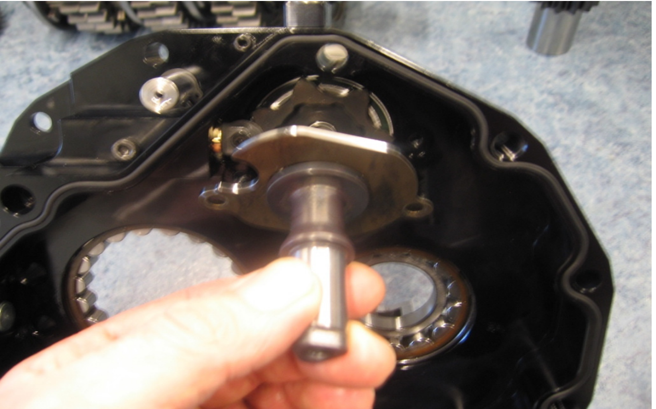
Remove the ratchet assembly
