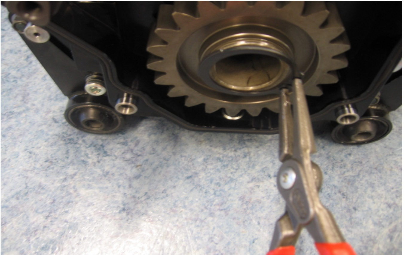
Fit circlip to lower drop gear, SGA40
