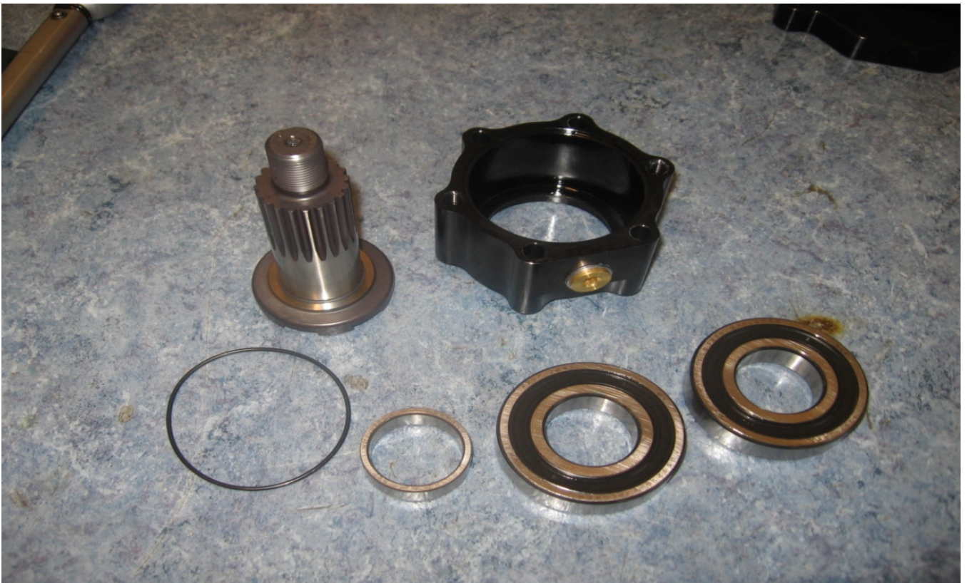
Press out the output shaft from the bearings
