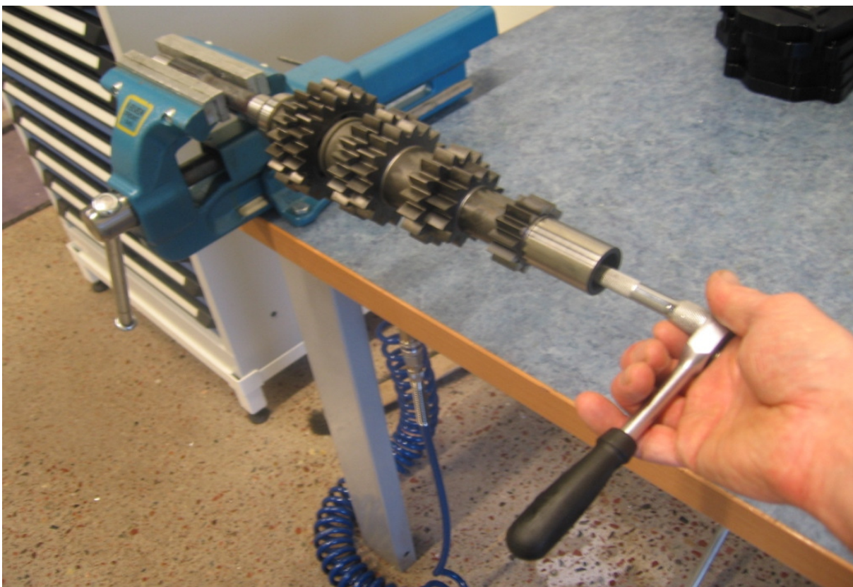
Remove the retaining bolt and top hat washer from clutch shaft. (Normal thread)
