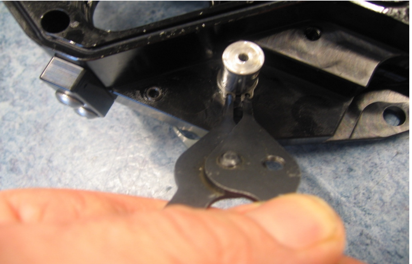
Remove circlip from neutral reverse axle.
